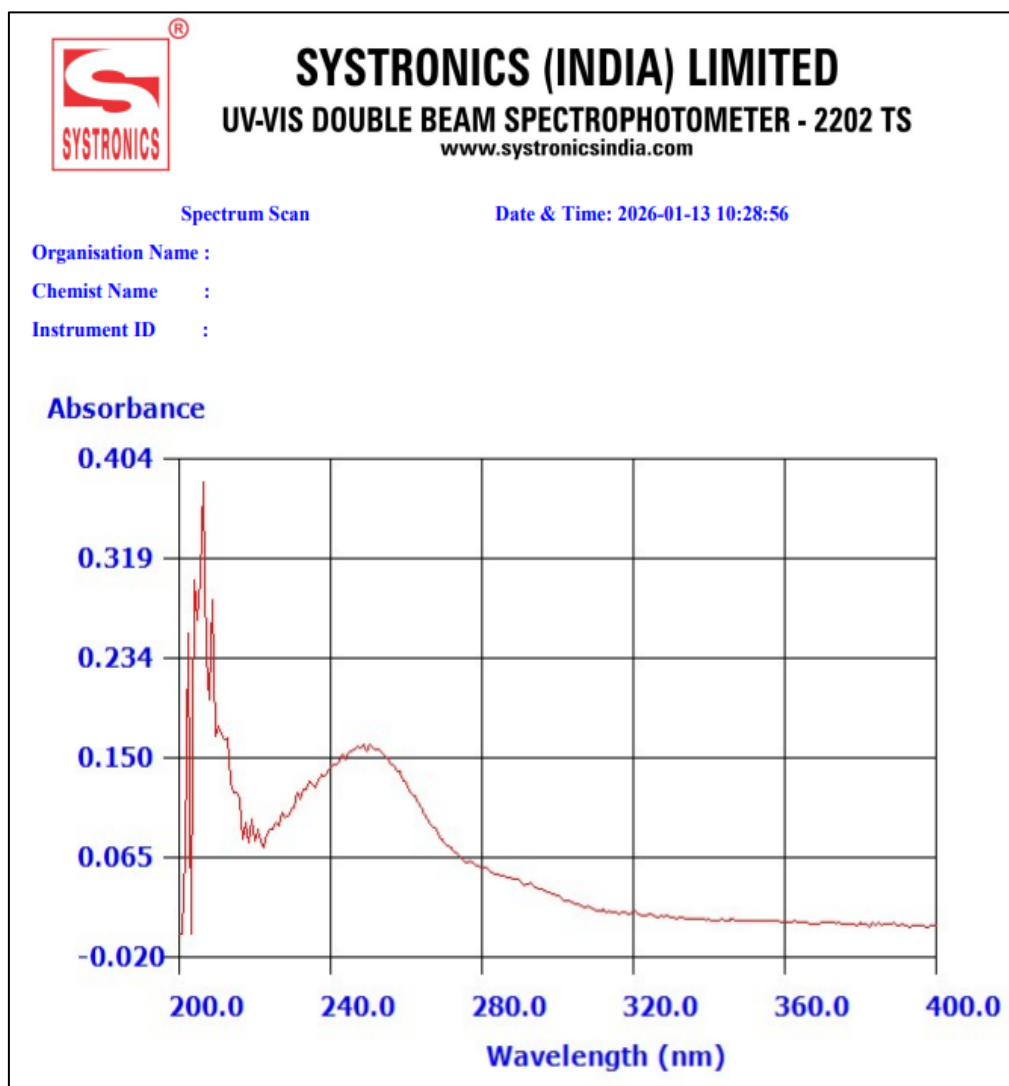
Fig 2 UV Spectrum of Itraconazole Showing the Reported Absorption Maximum at 264 nm
