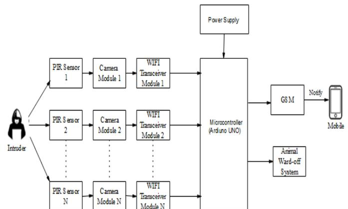
Fig.IoT Based Farm Intrusion Detection And Prevention System
