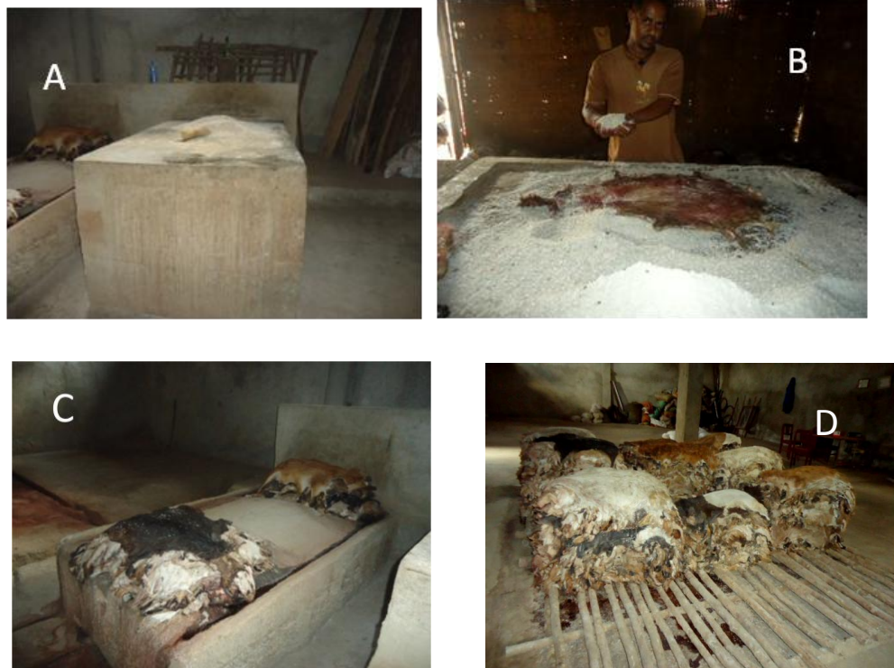
Figure 3: steps in curing of hides and skins
