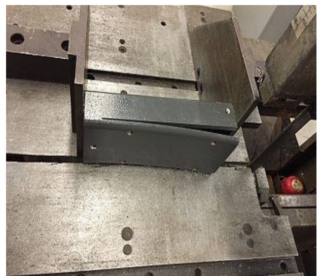
Fig1.4.1: Residual stress in a roll formed HSS tubing visible during band-saw slitting
