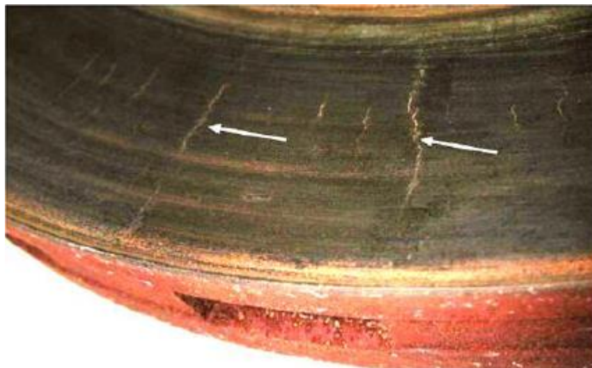
Fig.1.1.1 Thermal Cracking in Disc Brakes
