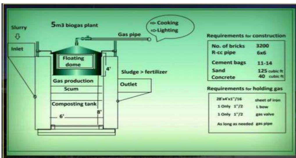
**Fig 10: Requirements for 5 m³ Biogas Plant**
