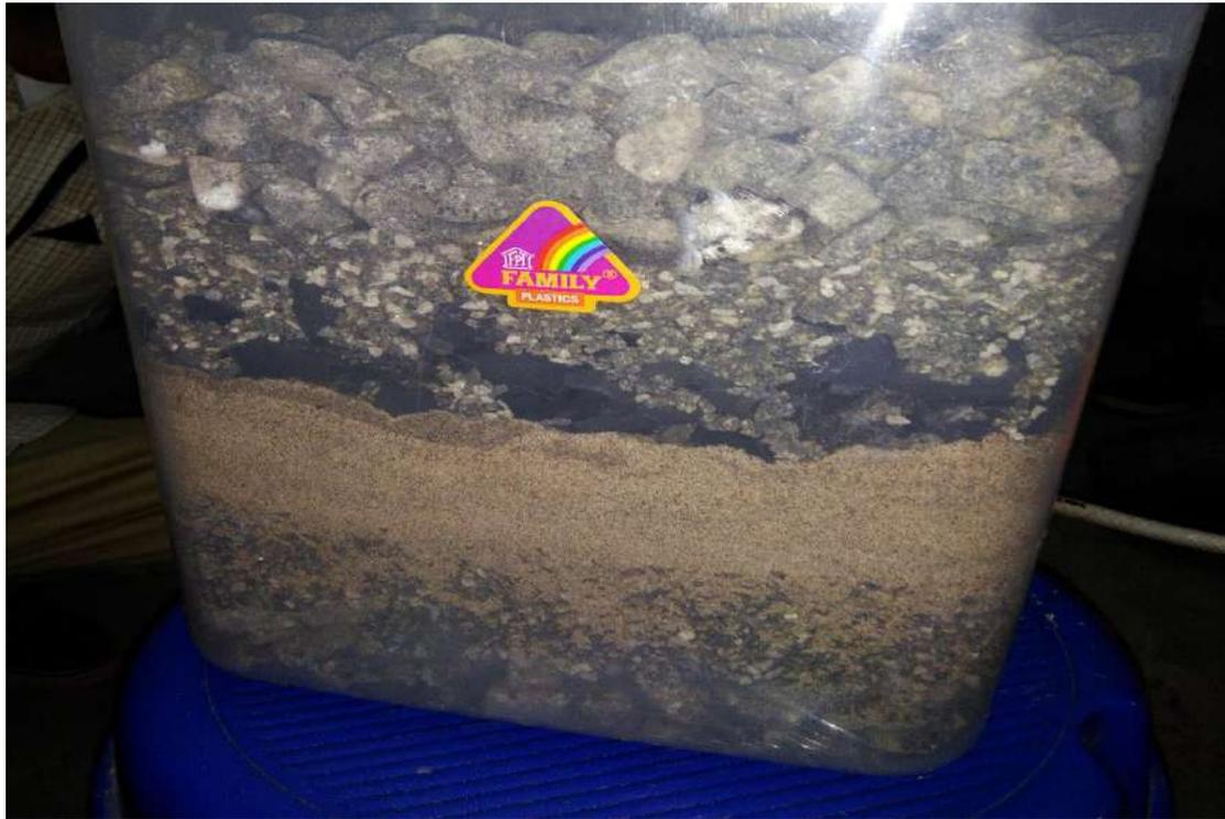
**Fig 13 (a): Layers of Filter**
