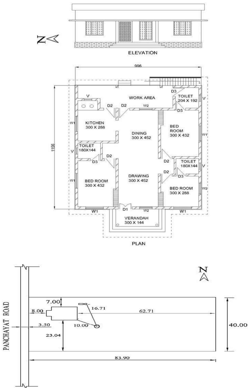
**Fig 4: Plan, Elevation and Site Plan of and Selected Building**
