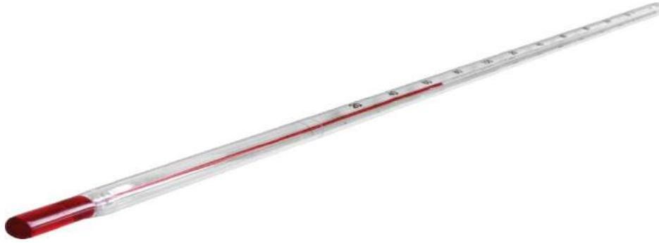
**Fig 5: Alcohol Thermometer**
