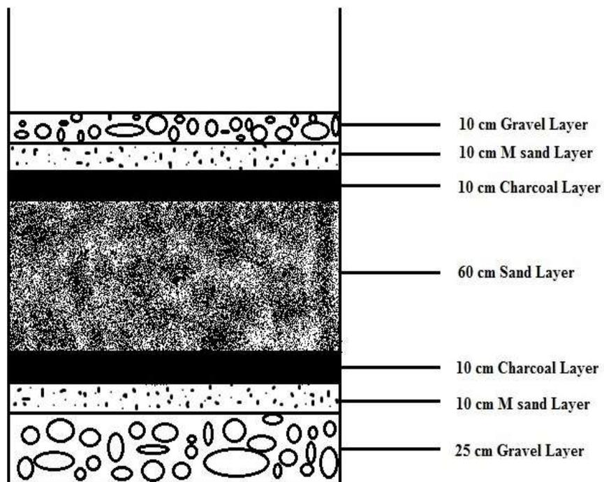
**Fig 13 (b): Thickness of each Layers in a Filter**
