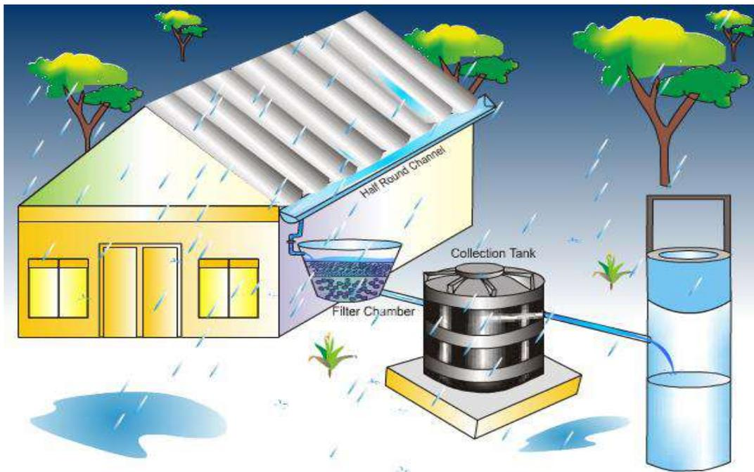
**Fig 7: Rain Water Collection in Asbestos Roofs**
