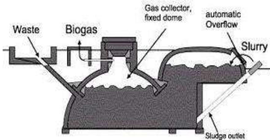
**Fig 9: Components of Biogas Plant**
