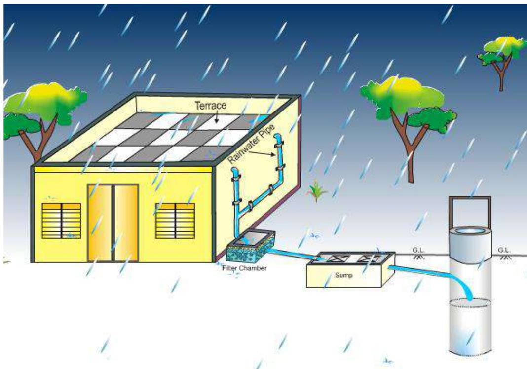
**Fig 8: Rain Water Collection in Flat Roofs**
