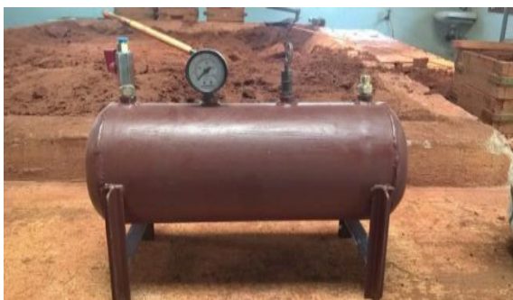
Fig 5.1.2 Air Storage tank
