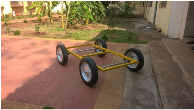
Fig 5.3.1 Frame of ms steel of 1.5inch welded as a frame using arc welding
