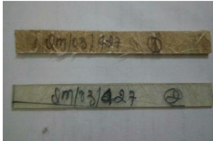
Fig4: Specimen used for Flexural Strength Test
