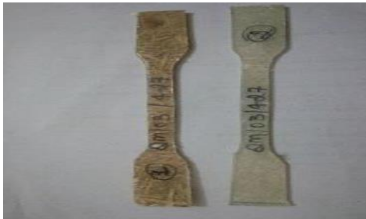
Fig 2: Specimen used for Tensile Strength Test
