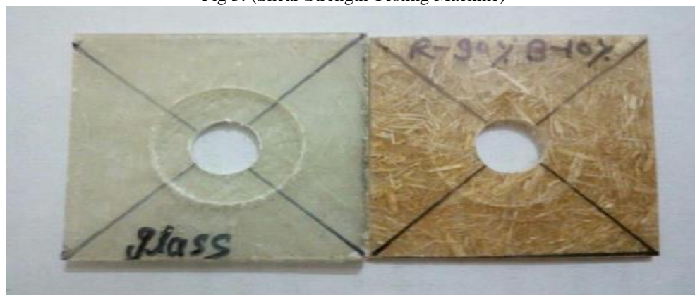
Fig 6: Specimen used for Shear Strength Test
