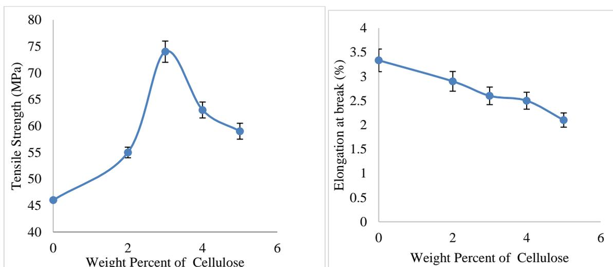
Cellulose of 2, 3, 4, 5 weight percents is incorporated in 2weight percent jute fiber reinforced polyester composite. The tensile strength of composites increased with respect to weight percent of cellulose upto 3 wt% and decreased with further increase in cellulose percent, further. The decline in tensile strength is due to agglomeration of nanocellulose and
