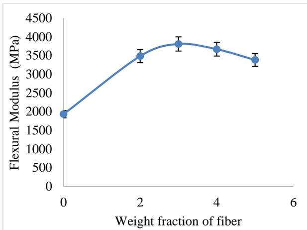
Flexural strength and flexural modulus 2weight percent of jute fiber based composite increased with increase in nanocellulose. The trend variation of flexural strength and flexural modulus is same. Highest flexural strength of 96MPa and flexural modulus of 3807MPa is observed at 3 weight percent of nanocellulose, which is due to good interference and adherence.
