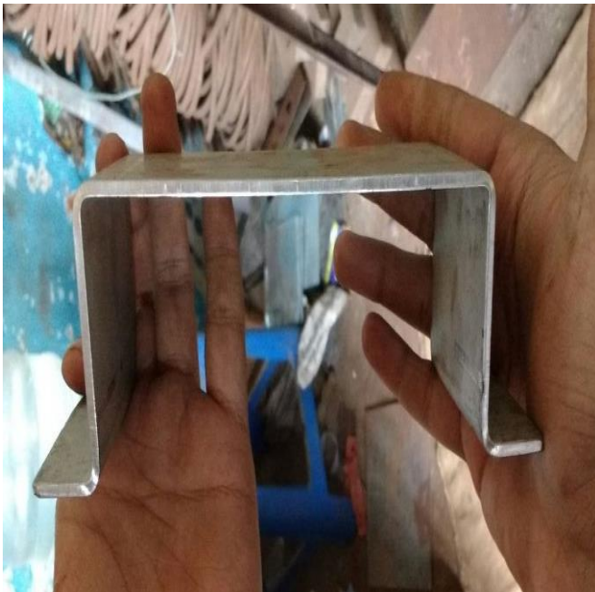
Fig 8. Bent Support Column Base
