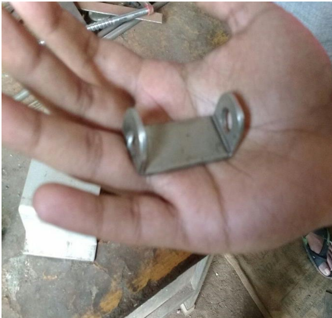
Fig7. Bent support strut of lathe rod
