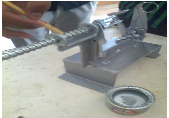
Fig 9. Fabricated Finished product – Anticorrosive Coating
