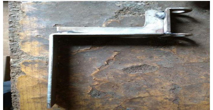
Fig.7:Support Base Strut (Fabrication)
