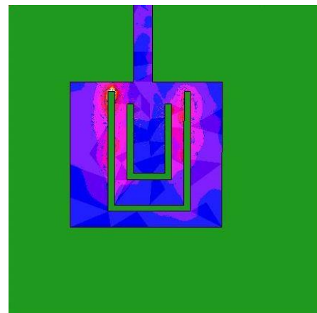
Fig 2.5 Simulated surface current distribution at (a) 2.75 GHz
