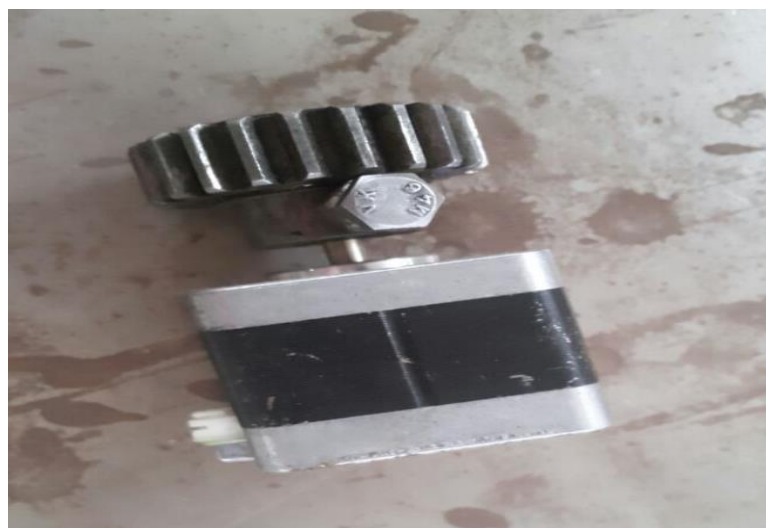
Fig. 3.5 Dynamo coupled with pinion gear
