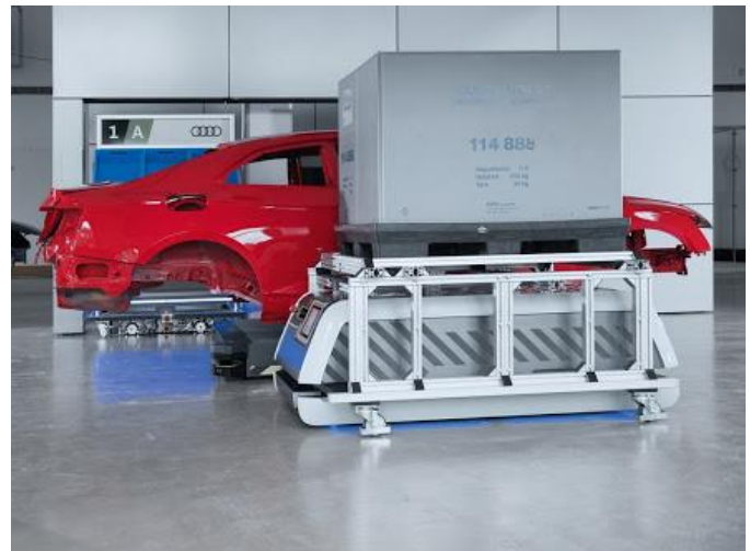
Fig. 3) – Audi AGV carrying load around the factory.
