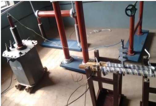
Figure 3: Setup for transformer to polymeric insulator
