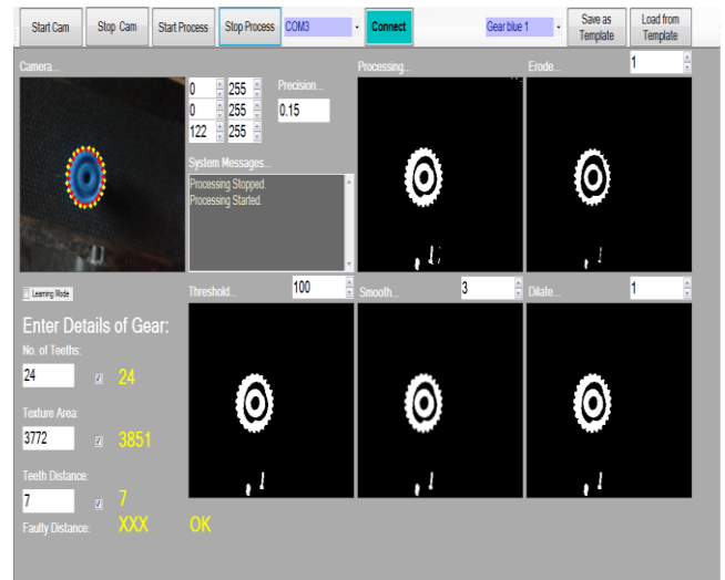
Fig 2: Non defective Gear
