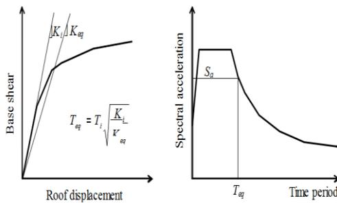
Figure 2 : Schematic representation of Displacement Coefficient Method (FEMA 356)
