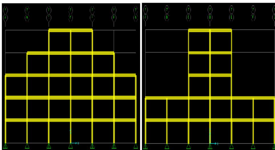
Figure 6 : Model 04 & 05 with 200% & 300% vertical irregularity
