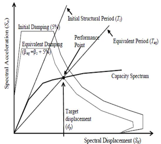
Figure 3 : Schematic representation of Capacity Spectrum Method(ATC40)
