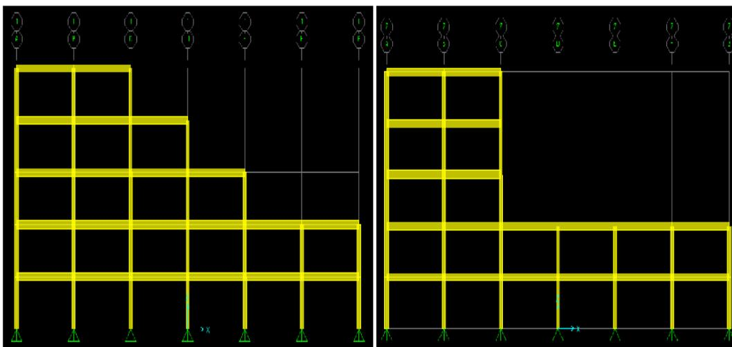
Figure 5 : Model 02 & 03 with 200% & 300% vertical irregularity
