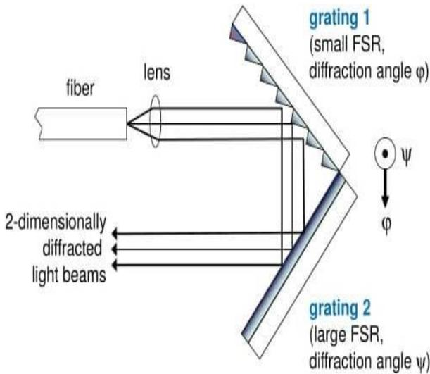
Fig.2 2D optical beam steering by a pair of crossed grating
