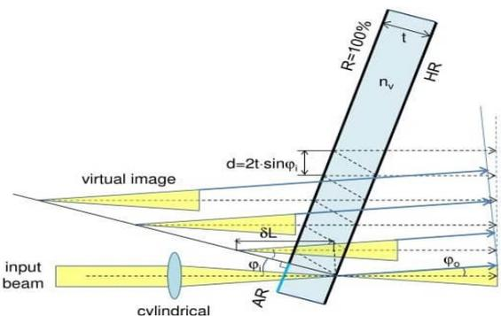
Fig.4 Virtually Imaged Phase Array
