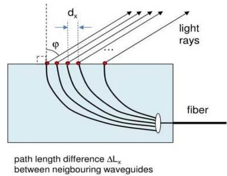
Fig. 3 Highly dispersive arrayed waveguide grating
