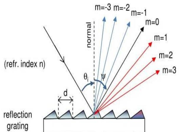
Fig.5 Reflection grating operating in various order m
