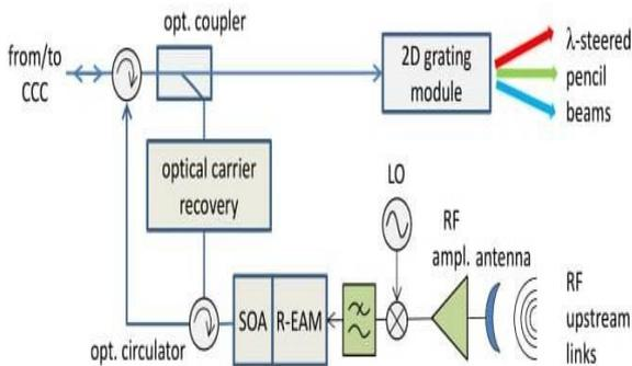
Fig. 6 Radio over fibre up steam path at PRA site, with optical carrier recovery
