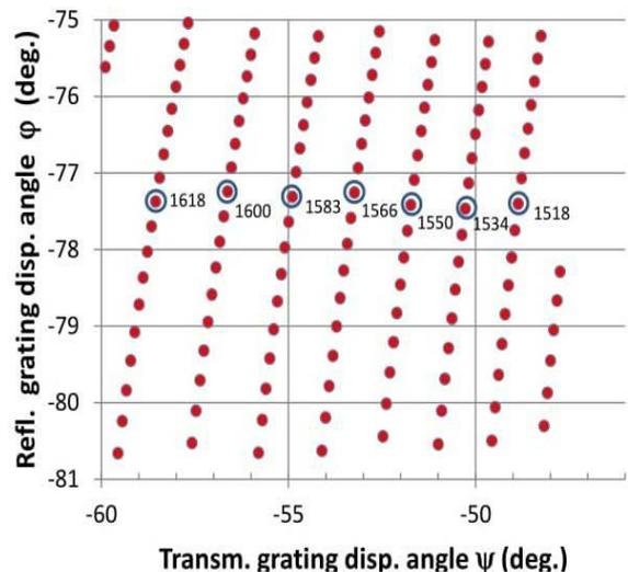
Fig. .8 2D beam scanning (simulated; encircled spots were measured at the wavelengths indicated)
