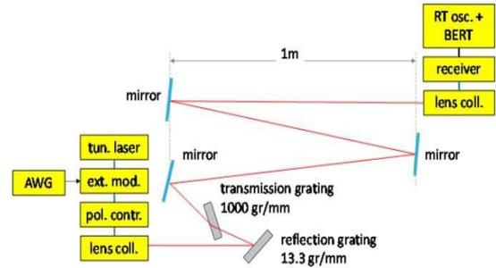
Fig. 7 2D beam-steered system experiment
