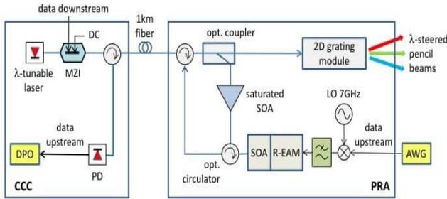
Fig. 9 Radio-over-fiber upstream system experiment
