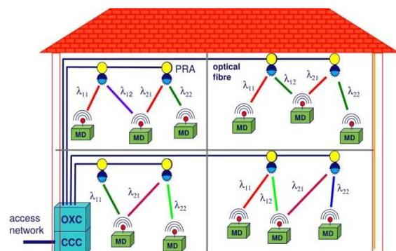
Fig.1 Free space indoor optical communication by pencil beam
