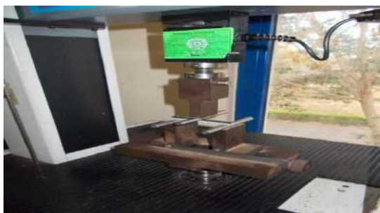
Fig 4 Equipment for Flexural Testing
