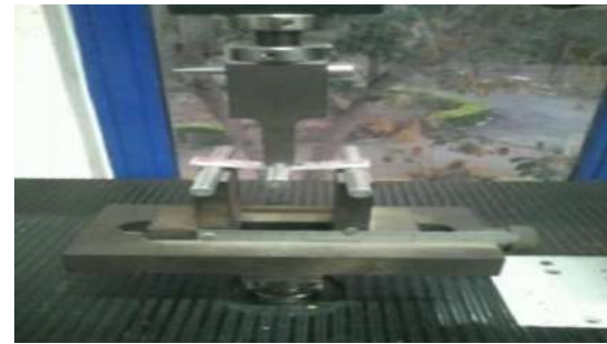
Fig 5 Loading Arrangement for Flexural Testing
