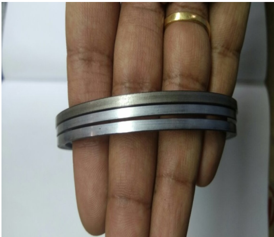
Fig 1.2: Piston rings after electroplating
