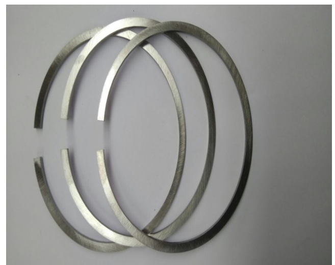
Fig 1.1: Piston Rings Before Electroplating
