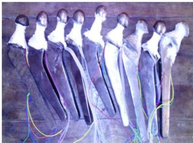
Fig. 4. Strain Gauges Attached At the Neck Region of the Nine Hip Implants.
