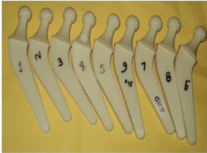
Figure 3. Nine Rapid prototyping patterns created From stl files of CAD models of the hip implant.
