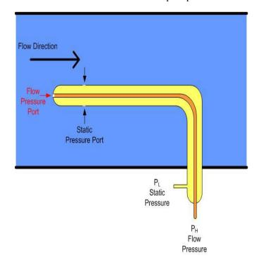
The above graph indicates how the Pitot tube is built of two tubes, one inside the other, to make a static weight port and a stream weight port. Applying Bernoulli's condition we get.
