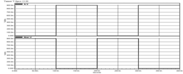
Figure 8: Input and output waveform of a NOT gate using modified GDI
