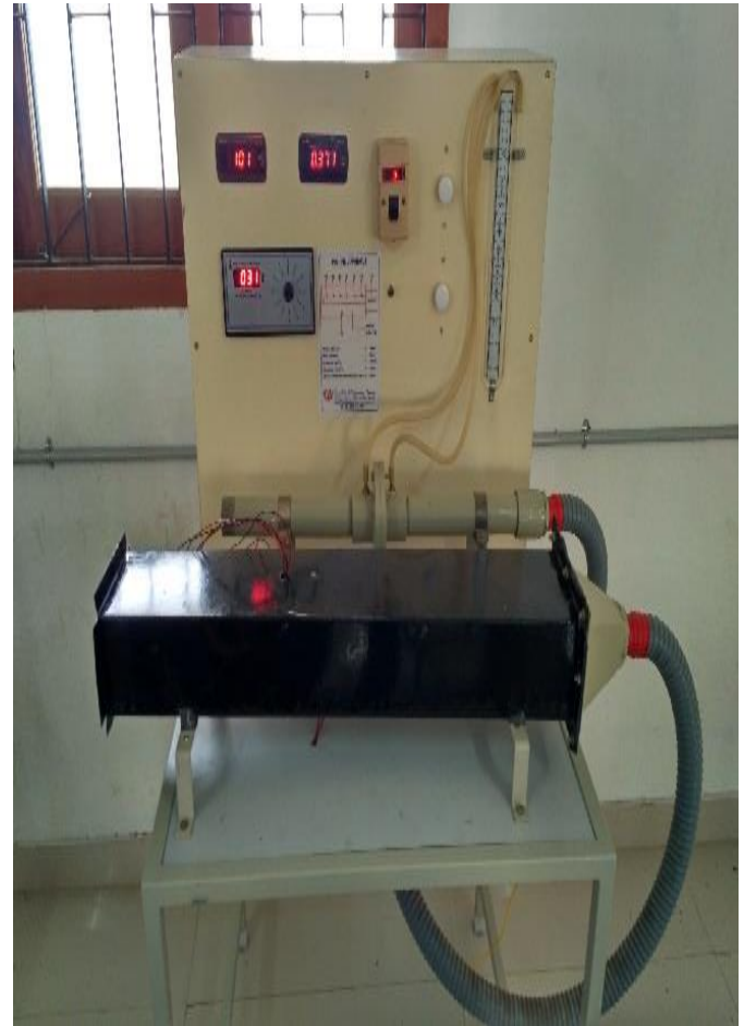
Fig 1 Experimental Setup For Pin Fin Apparatus
