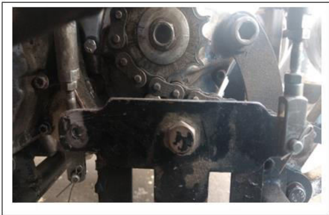
Fig.5: Plunger Rods Attached to Input Gear Lever of Gearbox (Front View).
