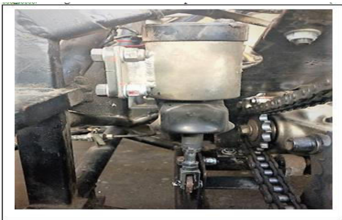
Fig. 6: Plunger Rods Attached to Input Gear Lever of Gearbox (Side View).
