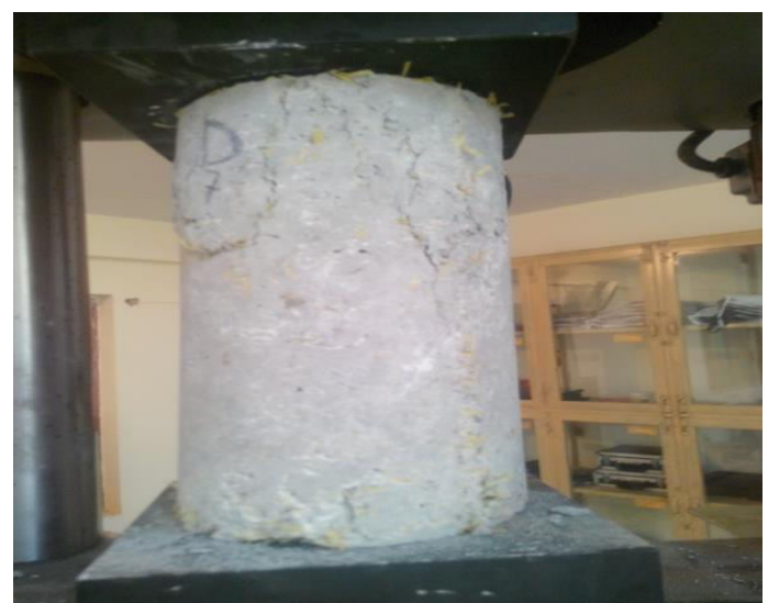
Figure: 4 Failure of PPFRC Under Compressive Load
