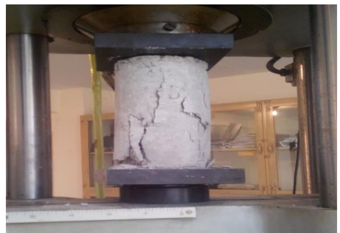
Figure: 3 Failure of Plain Concrete Under Compression
