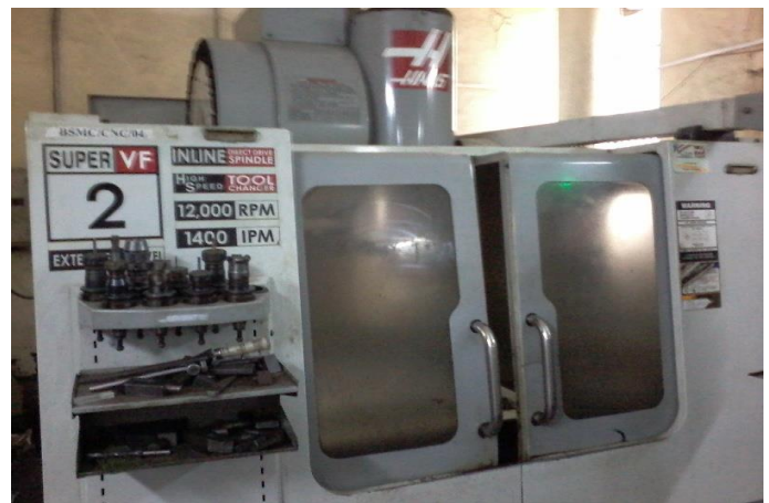
Fig. 1: CNC Vertical Machining Center (VMC) Model Super VF-2
