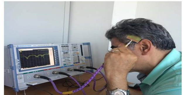
Fig 4: Measurement of the antenna on human’s head using network analyzer.
