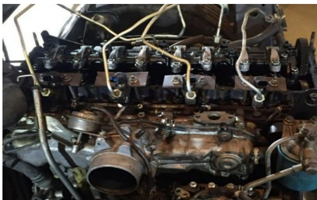
Fig 12. After Installing the Injectors
