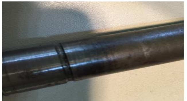
Fig 8. Injector after Grinding and Making Seal Groove
