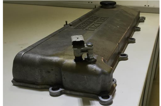
Fig 3. Cam Sensor Installation
