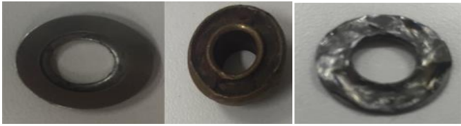
Fig 10. Machining of the Seat Ring Upper Face to Fit with the Old Seat
