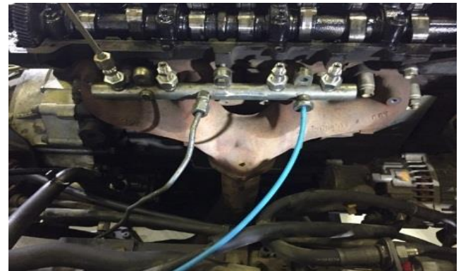
Fig 13. Installing Common Rail with Inlet and Return Pipes
