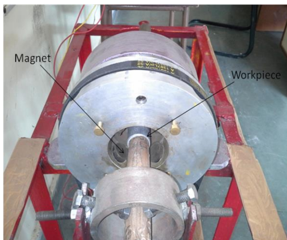
Fig. 3:- Magnetic chuck and work piece
