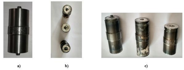
Fig. 2:- Tool Profile (a) New Tool (b&c) Pin broken and Deformed Metal sticks the tool shoulder
