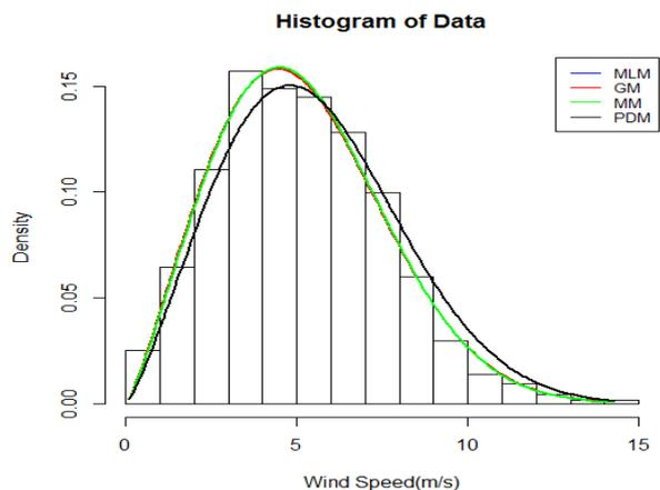
Fig 6:- Histogram of wind speed fitted with distribution methods
