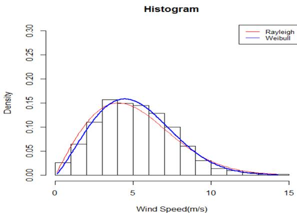
Fig 5:- Histogram of wind speed fitted with Rayleigh and Weibull curves
