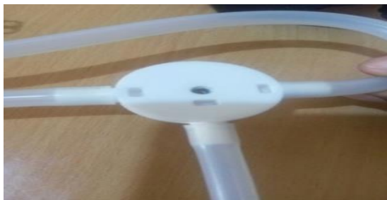
Fig 8:- Stator of Control Dial Valve
