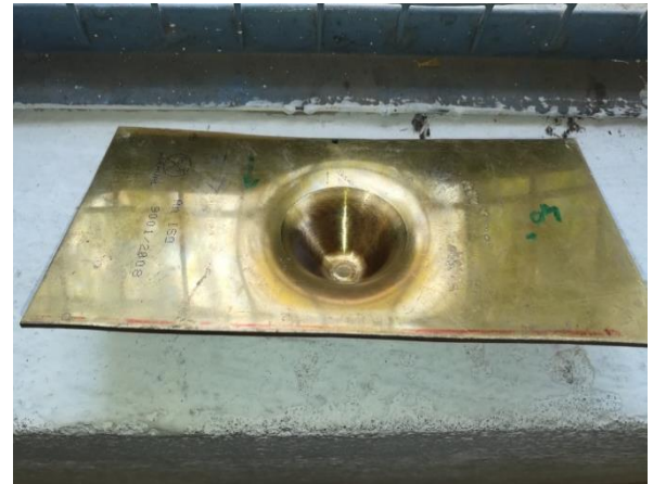
Fig 5:- Sample formed in cupping test
