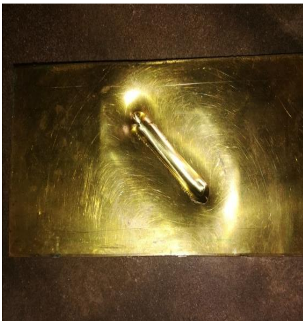
Fig 4:- Sample Formed in Straight Groove Test
