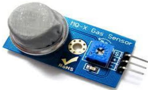
Fig 3:- MQ2 Gas Sensor
