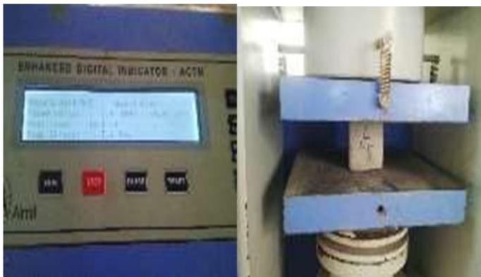
Fig 6:- compressive strength test
