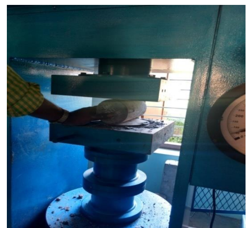
Fig 2:- Split strength check
