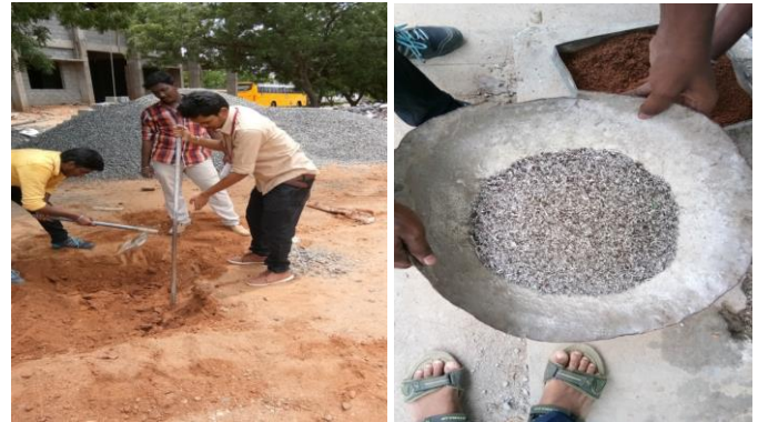
Fig 1:- Collection of Soil Samples and Steel Slag
