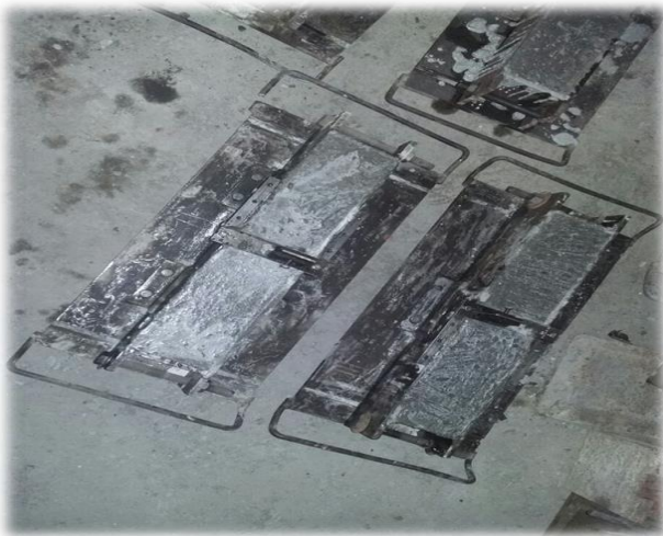
Fig 2:- Moulds of SENB Specimen
