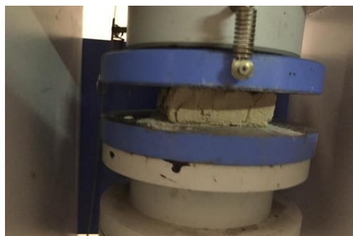
Fig 3.16 Compression testing on mycelium brick
