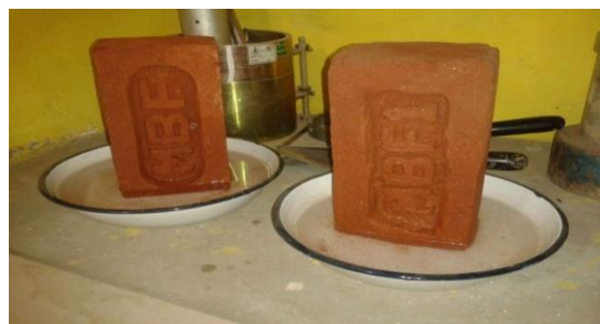
Figure A-2 Efflorescence test on bricks
