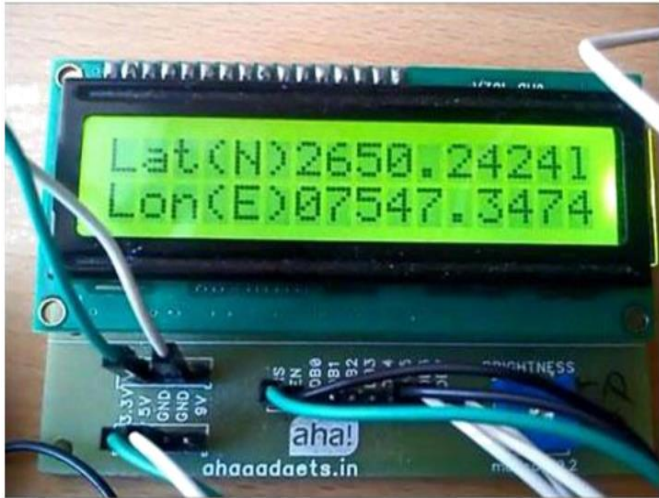
Fig 8:- showing latitudes and longitude values displayed on LCD
