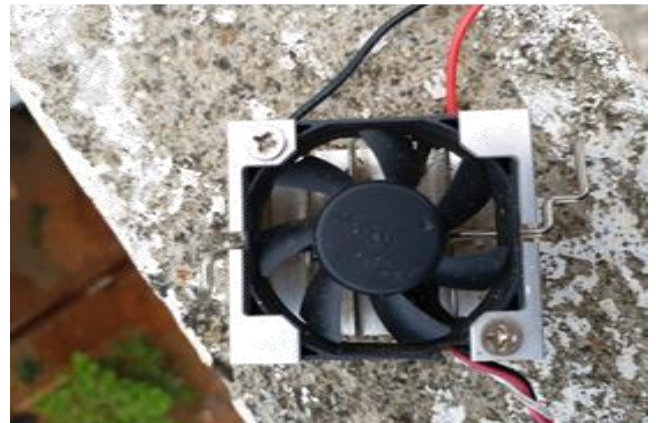
Fig 21:- Peltier module with Fan and heat sink
