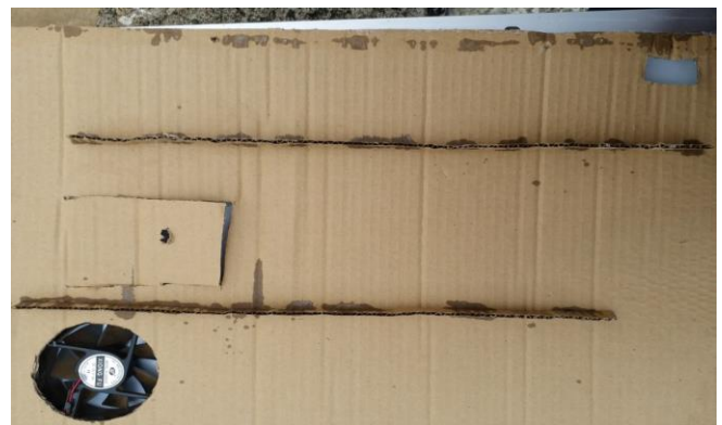
Fig 17:- Partition of air flow circulation
