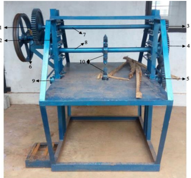
Gear 1, (2) Gear 2, (3) Gear 3, (4) Gear 4, (5) Gear 5, (6) Shaft 1, (7) Shaft 2, (8) Shaft 3, (9) Shaft 4, (10) Cutting Wheels
