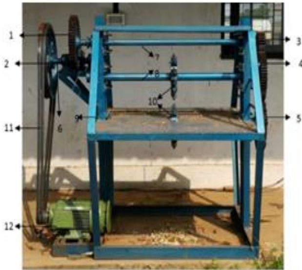
Gear 1, (2) Gear 2, (3) Gear 3, (4) Gear 4, (5) Gear 5, (6) Shaft 1, (7) Shaft 2, (8) Shaft 3, (9) Shaft 4, (10) Cutting Wheels
