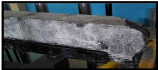
Fig 10:- Shear crack and failure at supports in specimen S2
