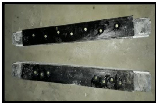
Fig 5:- Retrofitted specimens with steel channel and bolted connections
