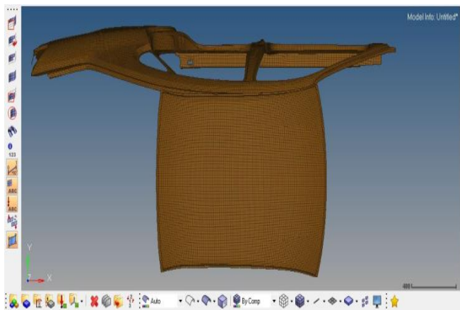
Fig 5:- Roof meshed part
