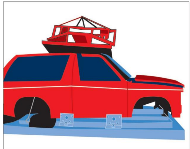
Fig 1:- FMVSS no 216 Test setup
