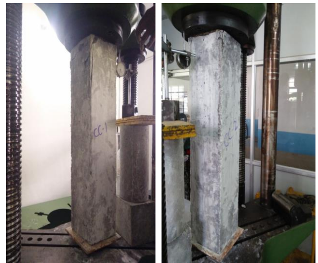
Fig 5:- Failure of convention columns
