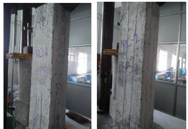
Fig 6:- Failure of type1 columns
