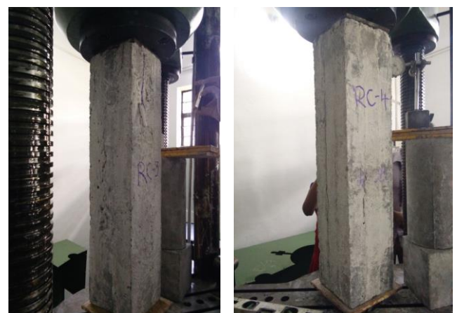
Fig 7:- Failure of type2 columns
