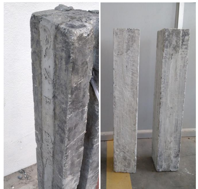
Fig 3:- Finished up specimens after retrofitting by providing covers
