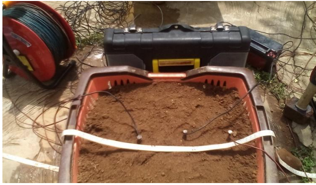
Fig 2:- a. showing the perforated basket during mechanical compaction b. showing the configuration for the dry sample while data is being acquired.
