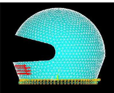
Fig 18:- Load applied on Chin portion
