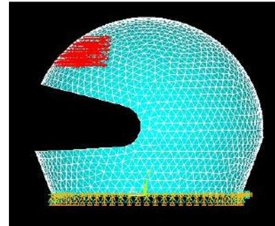
Fig 19:- Load applied on Fore Head portion
