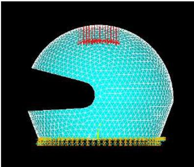
Fig 15:- Load applied on Top portion
