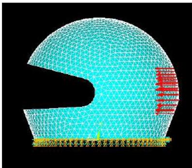
Fig 16:- Load applied on Rear portion
