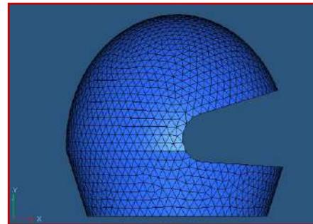
Fig 5:- Meshed model of helmet
