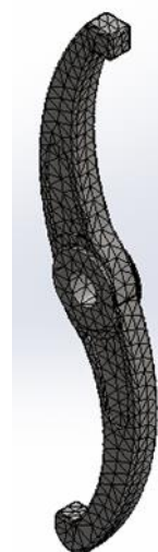
Fig 7:- Mesh model of the Puller handle
