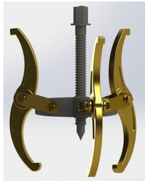
Fig 8:- The constructed Puller
