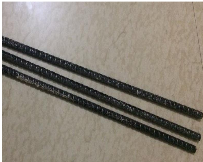
Fig 1:- Basalt fiber Reinforced Polymer Bar
