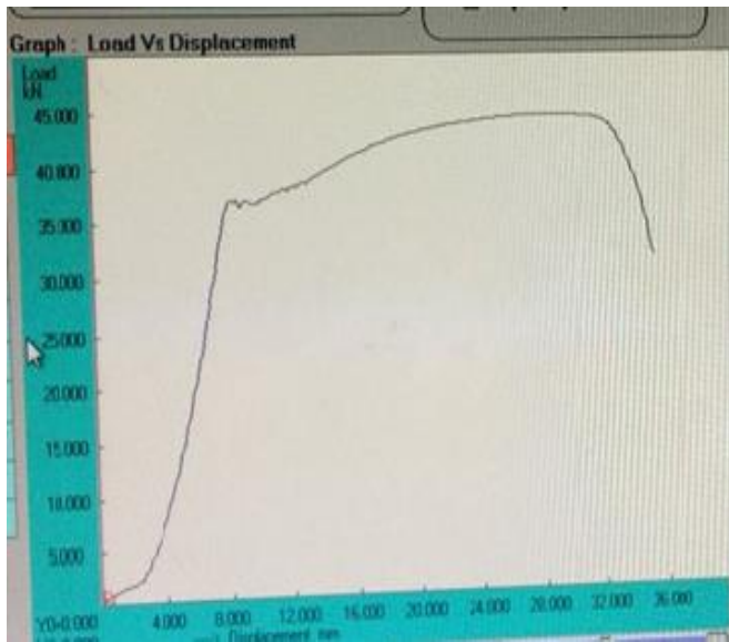
Fig 7:- Load- displacement curve of BFRP bar
