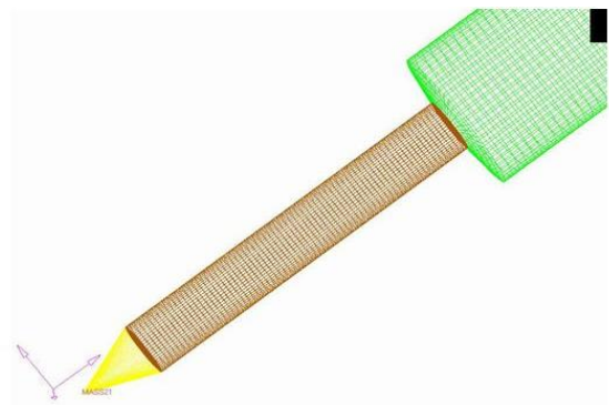
Fig 6:- Meshing of Spline Shaft and mass element
